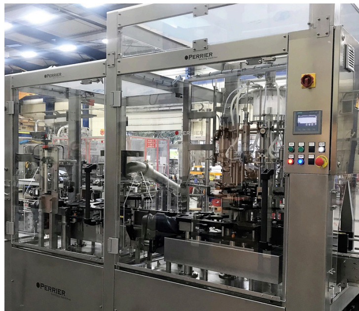
Disgorging and dosage rotating monobloc
