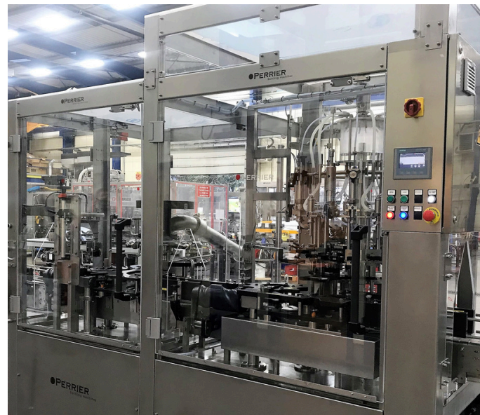
Disgorging and dosage rotating monobloc
